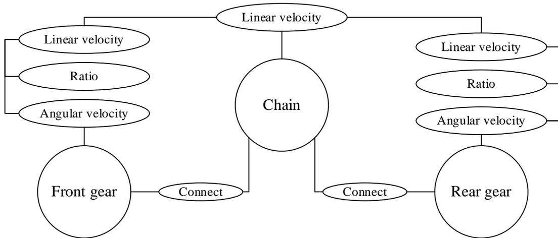
Figure 7. Bicycle transmission metamodel.
