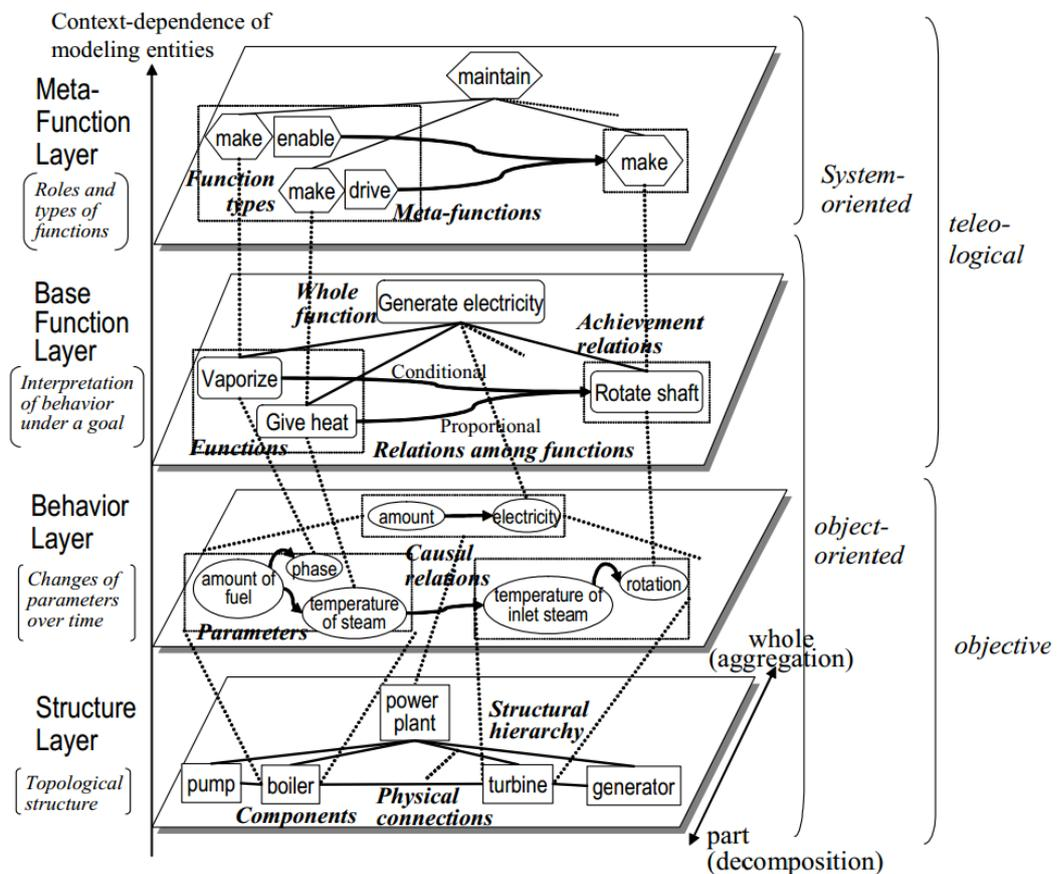
Figure 4. Hierarchy of a target object (power plant).
