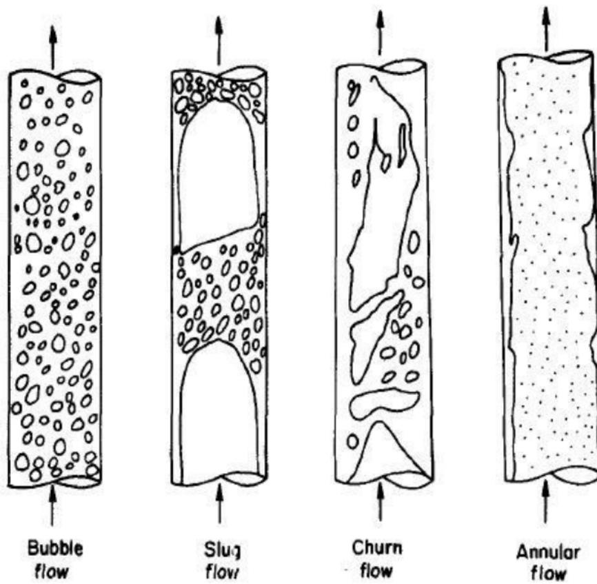
Figure 2: Flow patterns in vertical flow
