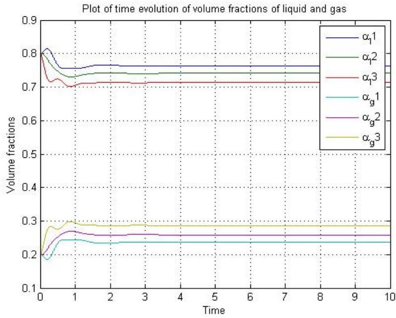
Figure 5: time evolution of volume fractions of liquid and gas
